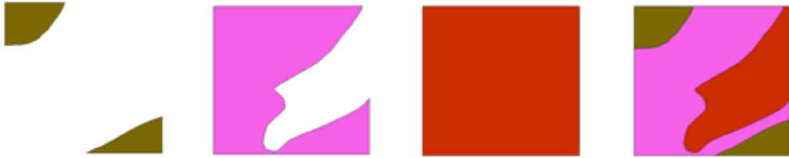
Left to right: Sandstone distribution map, Mudstone distribution map, Limestone distribution map, Composite map (i.e. geological map)
